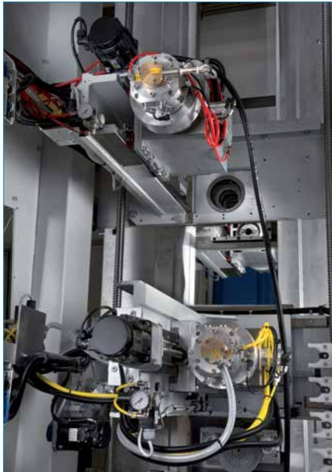
Processing with three heads, two for drilling and one dedicated head for milling, avoiding tool exchange when both processing types are executed.
