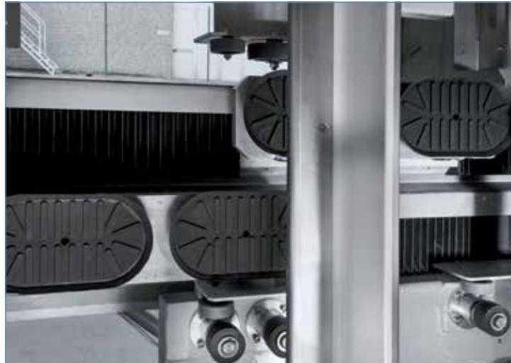
Conveying system with suction pads on the back side of the glass, never touching the glass on the frontal side, which makes it ideally suited for Low-E glass processing.
