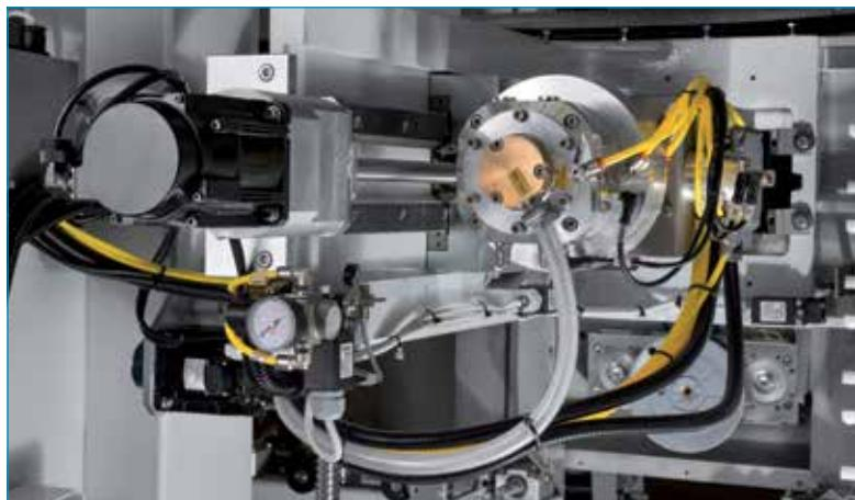
Three dedicated axes for the execution of notches with a dedicated head, with glass blocking by means of sucking pads positioned nearby the working area.
